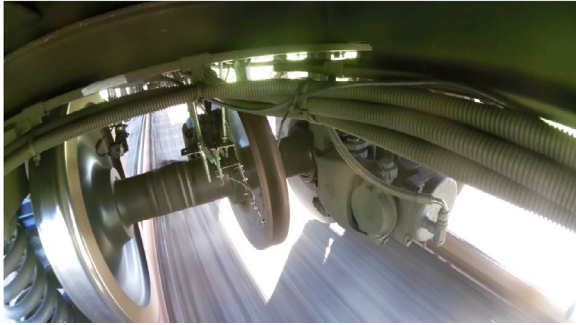
Disc in Green Cargo field test with measurement device
